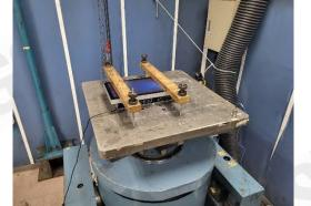
Functional Vibration Test: Z axis Operating Mechanical Shock Test: ±Z axis
